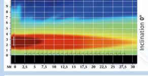
High sound pressure levels are confined within a band 1 to 4 m above the ground with good uniformity to approx.22m. Reflections from the ceiling are reduced, but reflections from the back wall are still probable
