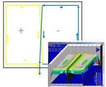
Figure 8 loops; easy to install. Provide good spill control in two direction. Provide moderate to good metal loss compensation.
