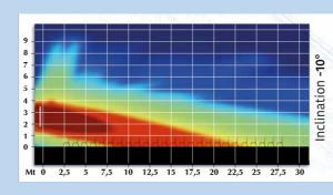
High sound pressure levels are confined within a 3m wide band and focused onto the congregation out to 22m. Now little energy is reaching the ceiling or rear wall so reflections are reduced and intelligibility is restored,
