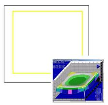
Perimeter loops; easy to install. Provide no compensation for metal loss. Spill field is 1 to 2 times the width of the loop To overcome this problem a delay is introduced between zones. Now the system is becoming quite complex! Each zone needs to be wired to a separate amplifier with a different (delayed) audio feed.
