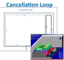
Cancellation loops; easy to install. Provide good spill control in 1 direction. Do not provide metal loss
