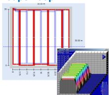
Superloop; moderately difficult to install. Provide good spill control in all directions. Provide good metal loss compensation. Excellent uniformity
